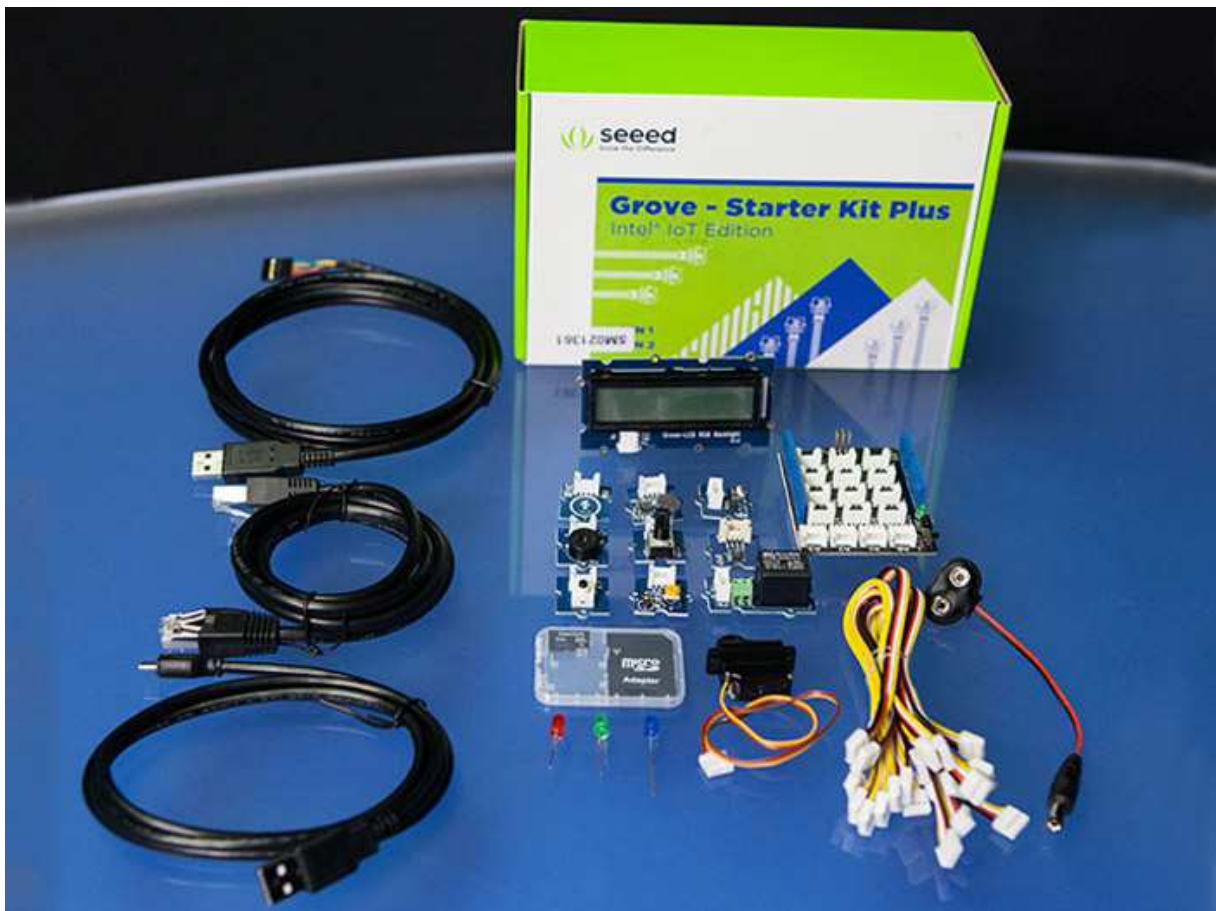
Fig.1. A set of sensors and wiring includes in Grove Starter Kit Plus Intel IoT Edition
